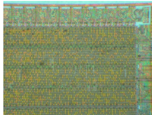
NEC \mu PD78F9116 microcontroller 0.35 \mu m
