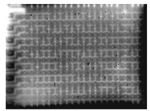
Motorola MC68HC705P6A microcontroller 1.2 µm
