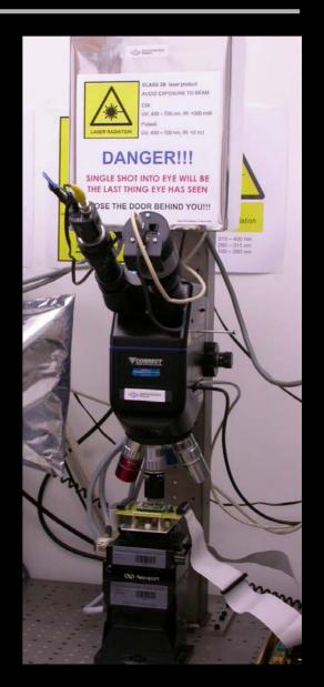
Experiments using Semiresearch Trioscan BSL2R special laser system for optical analysis of semiconductors
