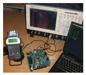
We constructed an FPGA design for capturing data
