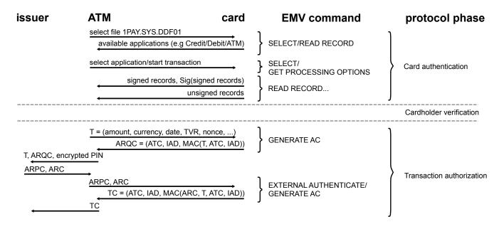
Figure 2. Outline of an EMV transaction at ATM. Note that while the messages between card and ATM have been verified, messages between issuer and ATM may vary depending on card scheme rules
