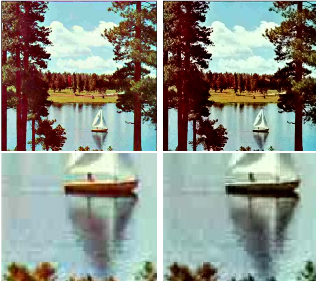
Fig. 13. Joint bilateral filter example. Left: JPEG compression using 2 \times 2 chrominance subsampling and IJG quality factor 20, file size 19,201 bytes. Right: JB-JPEG compression using 5 \times 5 chrominance subsampling, IJG quality factors of 22 for luminance and 75 for chrominance, file size 18,851 bytes. Joint bilateral filtering has prevented the colour shifts that are visible in the JPEG compressed image.
