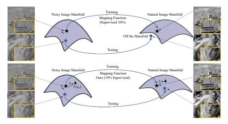
Fig. 2: The figure illustrates the mapping of image samples from noisy to original image manifold while training and testing. Model trained using only labeled data provides imperfect mapping resulting in reconstructed images lying off-the natural image manifold. Making use of large chunks of unlabeled data for training the same underlying model can provide a better mapping function. Best viewed when zoomed.
