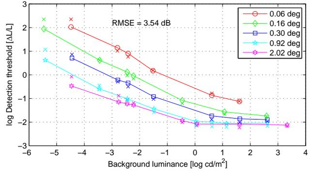
**Figure 9:** Visual model predictions for the **threshold versus intensity curve** data set. These are the detection thresholds for circular patterns of varying size on a uniform background field [Blackwell 1946].
