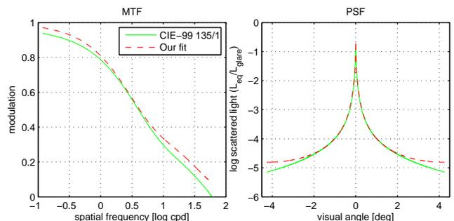
**Figure 3:** Comparison of our fitted intra-ocular light scatter model with the model from the CIE-99 135/1 report [Vos and van den Berg 1999]. Left panel shows the modulation transfer function of the eye and the right panel its corresponding point spread function. The MTF for the CIE-99 135/1 glare spread function has been computed by creating a densely sampled digital filter and applying the inverse Fourier transform.
