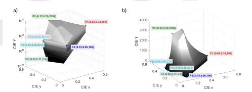
Fig. 7. a) 3D colour gamut in CIE xyY chromaticity coordinates, plotted in log scale for the luminance axis. b) 3D colour gamut as in (a), shown again here in CIE xyY chromaticity coordinates, in linear scale for the luminance axis. These figures are also provided as movie files in Visualization 1 and Visualization 2.
