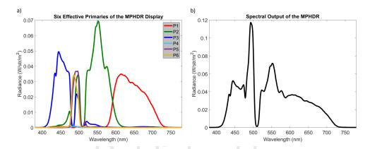
Fig. 4. a) The six effective primaries available from the MPHDR display. Note, the spectra of primaries,  $P_4(\lambda)$ ,  $P_5(\lambda)$ , and  $P_6(\lambda)$ , are measured from 380 nm to 560 nm given the transmission properties of the bandpass cut-off filter placed in the top HDR configuration. b) The spectral output of the MPHDR display when all six effective primaries are set to maximum.
