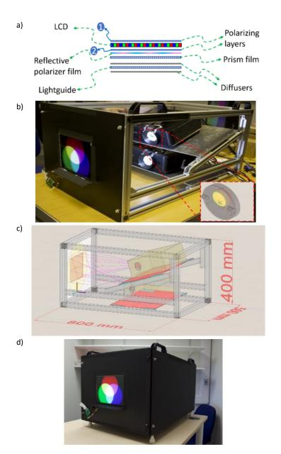
Fig. 3. a) Layers of a generic LCD panel. b) Photograph of the MPHDR without the final casing. The CAD design of one of the 3D printed filter mounts is shown as an inset. c) A representative CAD drawing of the setup. d) Photograph of the MPHDR with final casing.
