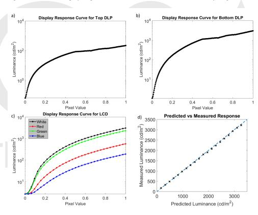
Fig. 5. a) The display response curve for the top projector. b) The display response curve for the bottom projector. c) The display response curve for the LCD panel. d) Predicted and measured luminances (black cross symbols) match after display response correction.
