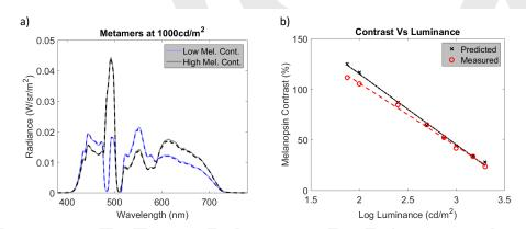
Fig. 8. a) An example of a metameric pair of melanopsin isolating stimuli. The measured spectral output from the MPHDR display (shown as a dashed line) overlaps the desired spectral output from the MPHDR display
