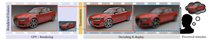
Figure 1: Our technique renders every second frame at a lower resolution to save on rendering time and data transmission bandwidth. Before the frames are displayed, the low resolution frames are upsampled and high-resolution frames are compensated for the lost information. When such a sequence is viewed at a high frame rate, the frames are perceived as though they were rendered at full resolution.
