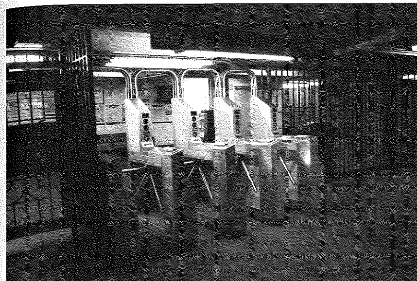
Figure 8. Contemporary turnstile with sloped side panels and other features to ward off fare beating. Photo by Noah McClain.
