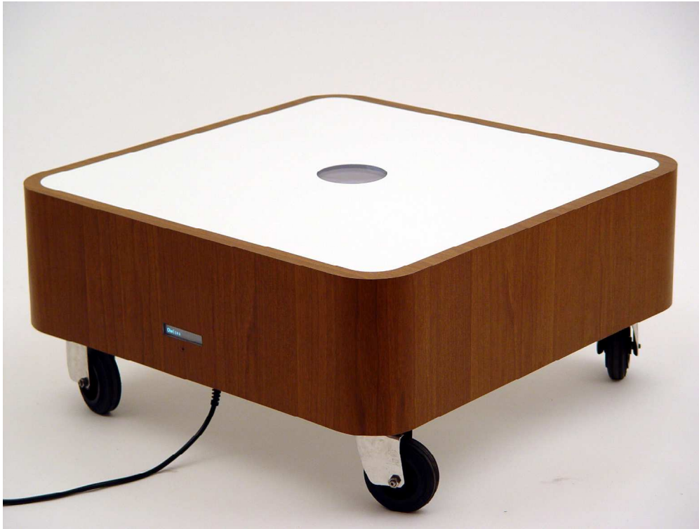
The Drift Table shows slowly scrolling aerial photography through the viewport on its top. 903x677mm (600 x 600 DPI)
