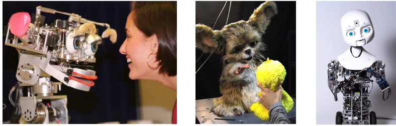
Figure 1: Three examples of social robots used in this research: Kismet (left), Leonardo (center), and Nexi (right).
