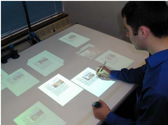
Fig. 2. The Escritoire is a desk-sized display on which items like documents and images can be manipulated.
