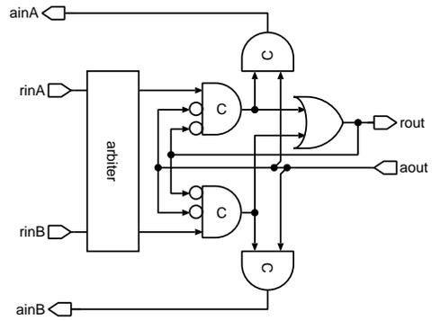
**Figure 5. 4-phase call element with arbitration**
