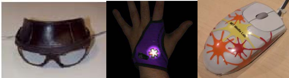
Figure 6 Affect sensing technologies: (left to right) The Expression Glasses [55], the Galvactivator [44], the Pressure Mouse [49]
