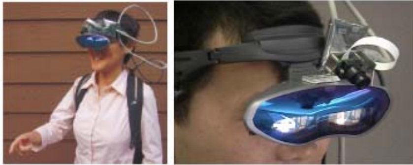
Figure 8 Mobile user interface used in Kolsch et al [31]. All hardware components aside from display, camera, and microphone are in the backpack.
