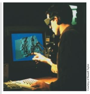
5 View of UNC nanoManipulator connected to an atomic force microscope.
