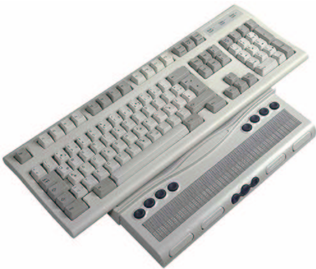
Fig. 1 A refreshable Braille display attached to a normal keyboard (photograph from www.tieman.de )
