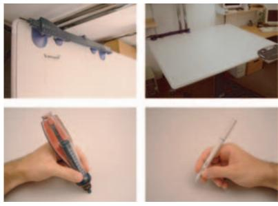
Figure 3. We combined (bottom left) an ultrasonic pen and (top left) its receiver bar with (top right) a large digitizer and (bottom right) its pen. The receiver bar attaches horizontally to the digitizer's back edge.
