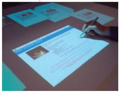
Figure 4. Web browser being accessed through Virtual Network Computing and placed on the desk with other documents.
