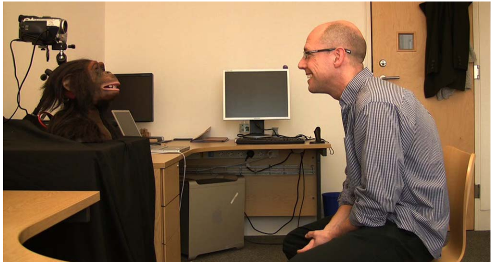
Fig. 3 The experimental setup. A participant sits in a chair facing the robot, about one meter away from it. The camera and chair position remain fixed across all participants
