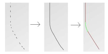
Figure 2. The three phases of fragmentation. A continuous curve is obtained by connecting line segments with Bézier curves. Then, the entire stroke is segmented into linear curved segments using its global properties.
