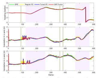
Fig. 4. Plots of heading and translation of host vehicle at each frame
