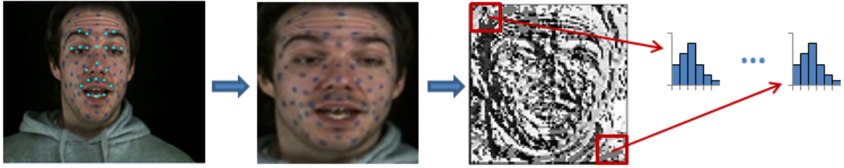
Figure 1: The extraction of linear binary patterns from an image to construct features for video emotion classification.
