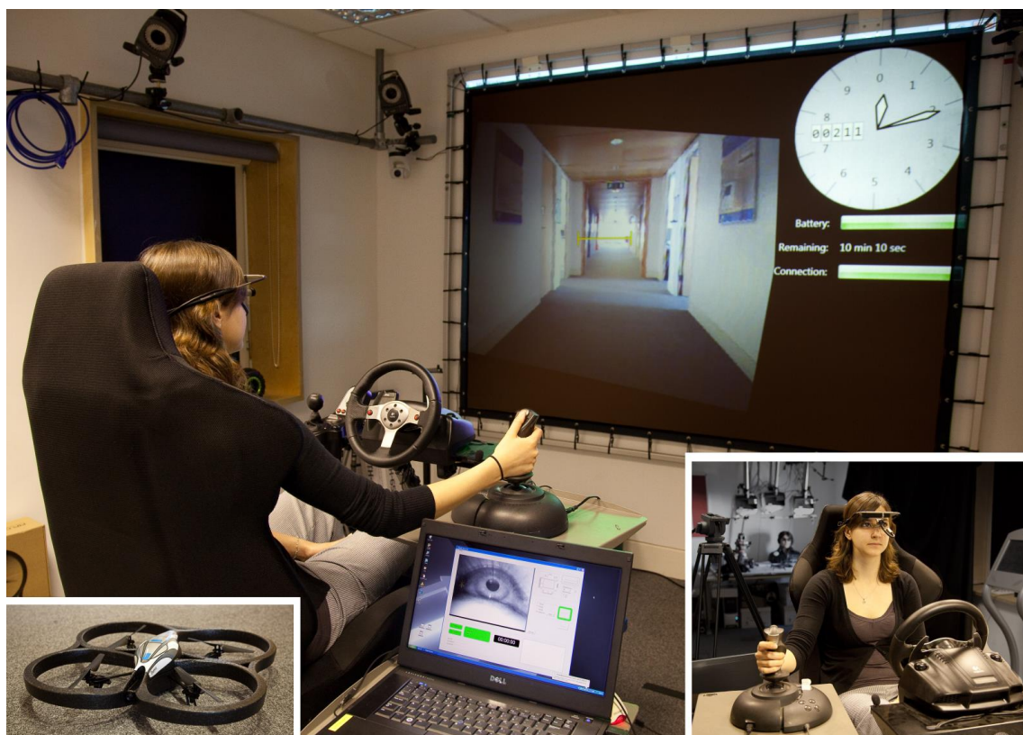
Figure 3: A simulator to investigate drivers' signs of cognitive overload
