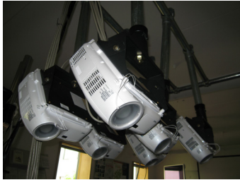
Figure 4: The T3 projected tabletop display.
