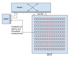
Fig. 2. SNT - Traffic amplification & flow monitoring
