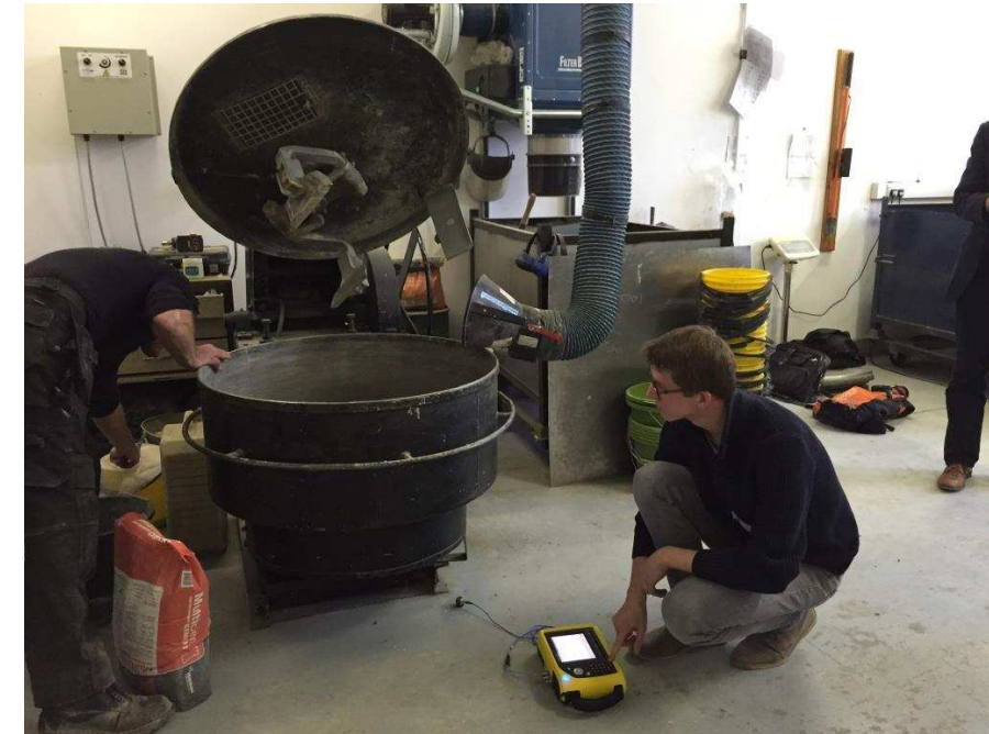
Figure 1: Concrete Mixer under test
