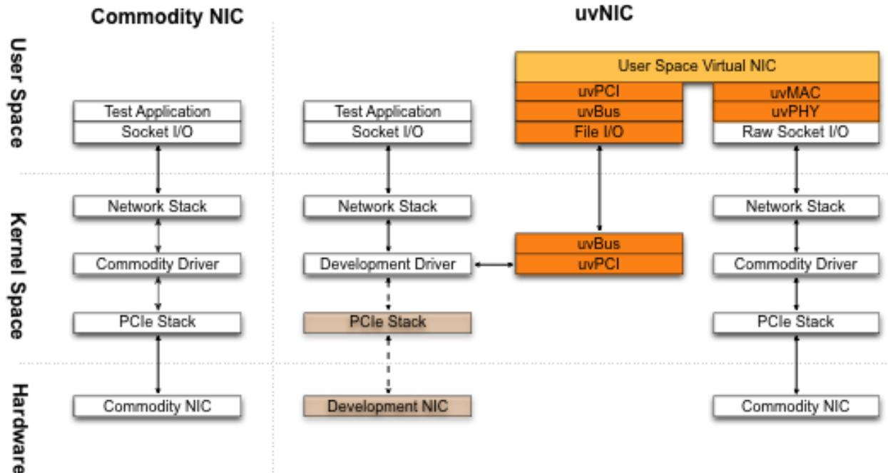
**Figure 1a - Arrangement of a typical network interface controller (NIC) hardware and driver; Figure 1b - Arrangement of a the uvNIC driver, virtual PCIe bus, virtual hardware and underlying hardware.**
