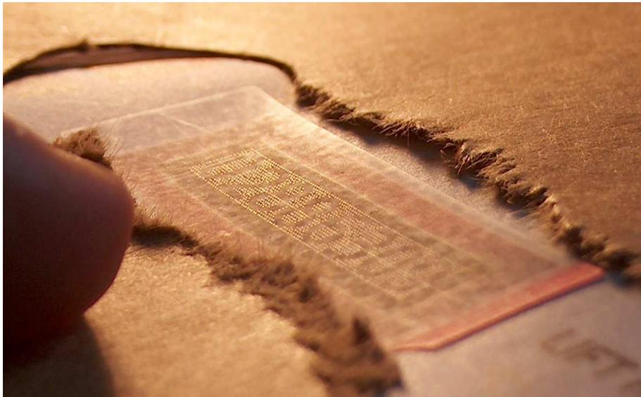
**Fig. 5.** Angled Light Attack on PINTAB Mailer (Nominet UK, Jun 2005), brown envelope mask used to reduce glare for purposes of photography
