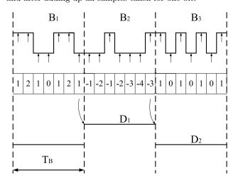
Figure 5: Example of majority voting over a bit period. Here the receiver samples the incoming signal  $B_{1,2,3}$  seven times during each bit period  $T_B$ . It then decides, based on the vote, whether to make the corresponding output  $D_{1,2}$  high or low.
