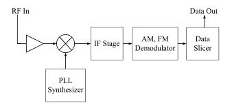
Figure 3: Functional diagram of a generic superheterodyne RF receiver
