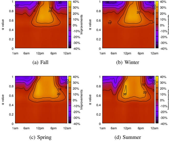
Fig. 7: Improvements of brown energy saving over shortest path (OSPF) *rePGBR* exhibits between -40% and 40% energy saving improvements when compared to using only shortest path. The values of  $\alpha$  resulting in high improvements are numerous and predictable.
