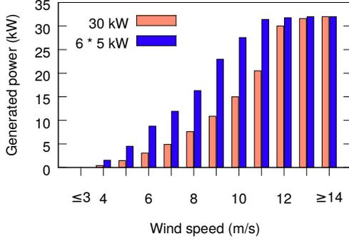
Fig. 4: **Wind speed to power conversion** Using smaller wind turbines for the distributed renewable infrastructure is more advantageous than their larger counterparts. The wind speed to power conversion is obtained from [16].
