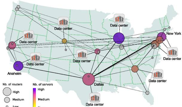
Fig. 1: **Sprintlink USA mainland network** [14]. The ISP network used in the evaluation of our proposed solution. The size of the bubbles indicates the size of the POP. The placement of data centers is explained in Section V-A.
