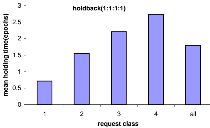
Figure 6: Mean holding time of each class for holdback(1:1:1:1) (M=0, N=16)
