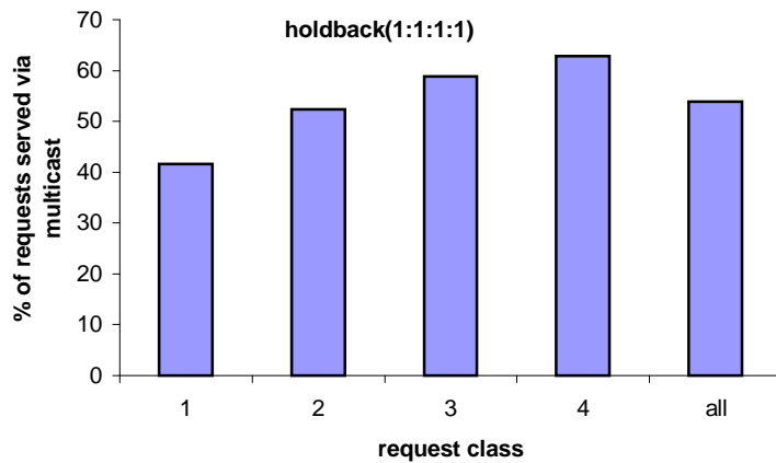
Figure 7: % of each request class served via multicast with holdback(1:1:1:1) (M=0, N=16)
