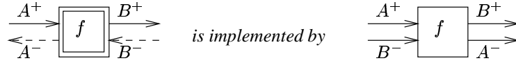
Fig. 6. A process with bi-directional I/O implemented by an uni-directional process. Dotted lines indicate channels that play the opposite role in the higher-order model
