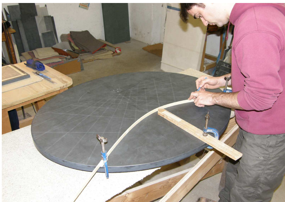
Fig. 6 — Russell Purdham setting out the Summer Solstice Curve
