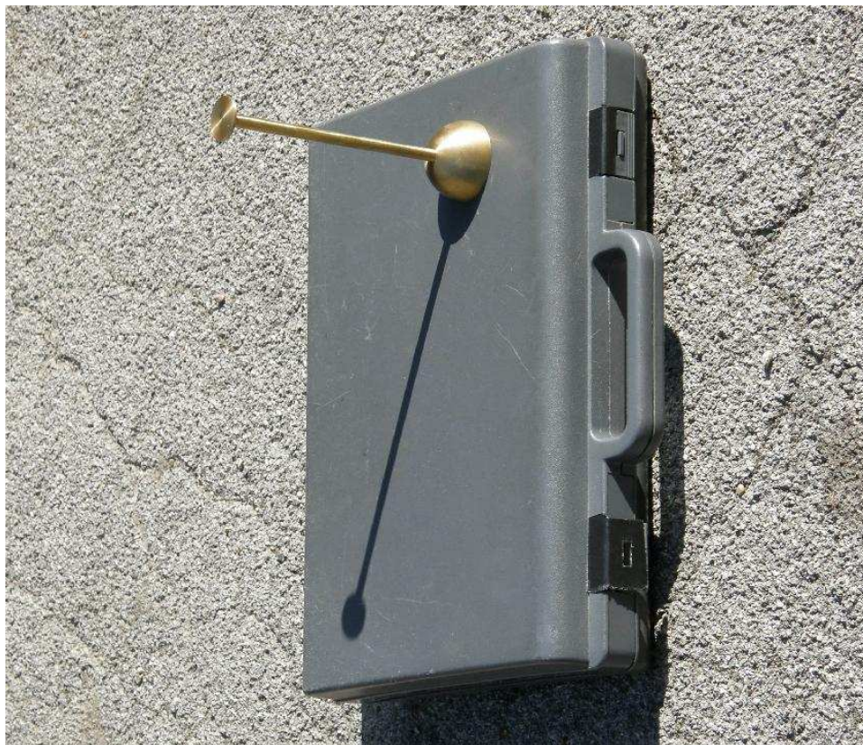
Fig. 2 — The Nodus and Nodus Support
