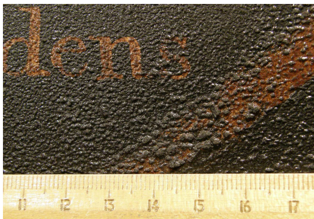
Fig. 8 — Example of Serious Alligatoring
