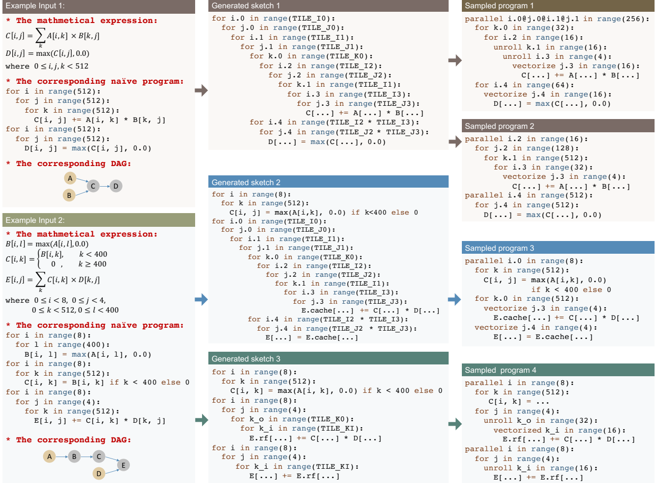
Figure 5: Examples of generated sketches and sampled programs. This figure shows two example inputs, three generated sketches and four sampled programs.
