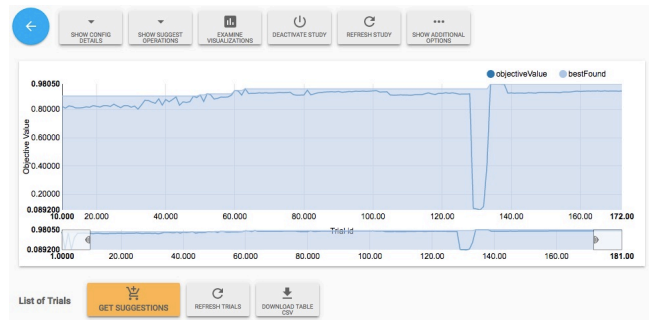
Figure 3: A section of the dashboard for tracking the progress of Trials and the corresponding objective function values. Note also, the presence of actions buttons such as Get Suggestions for manually requesting suggestions.
