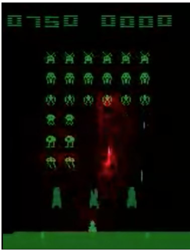
Fig. 5. Saliency map of a trained DQN [71] playing “Space Invaders” [8]. By backpropagating the training signal to the image space, it is possible to see what a neural-network-based agent is attending to. In this frame, the most salient points—shown with the red overlay—are the laser that the agent recently fired, and also the enemy that it anticipates hitting in a few time steps.
