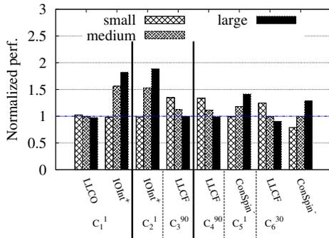
**Figure 7. The benefit of quantum length customization:** This figure shows that even if the clustering step improves applications’ performance, performance can be further improved by quantum length customization. The results are normalized over the performance when both clustering and quantum length customization steps are activated.
