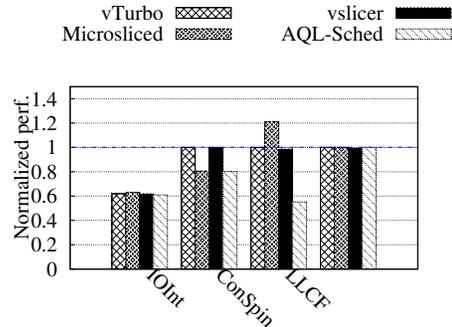
**Figure 8. Comparison with other systems:** This figure presents the comparison results of our prototype (*AQL\_Sched*) with vTurbo, vSlicer, and Microsliced. These results are normalized over the performance obtained with the default Xen scheduler.
