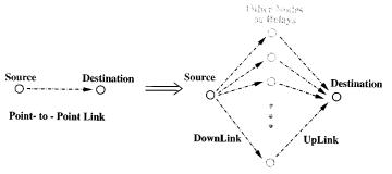
C. Mobile nodes with relaying: throughput of O(1)
