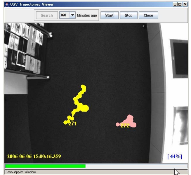
Figure 7: A snapshot of the human trajectory viewer. It shows two stored trajectories retrieved from the system. In the figure, a trajectory at the right side shows a man has been staying there. The other shows a man has been moving through the center area.
