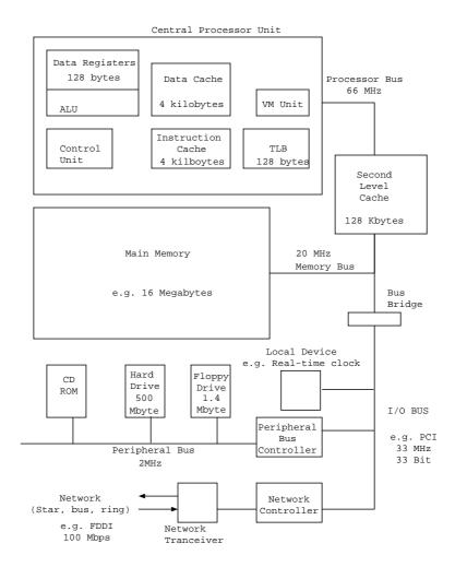
Figure 9.1: A system with multiple busses
