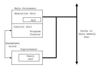
Figure 6.1: Coprocessor Typical Configuration
