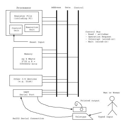
Figure 1.1: Simple Von Neumann Computer Architecture
