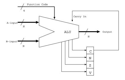
Figure 1.2: Usual configuration of flags with an ALU
