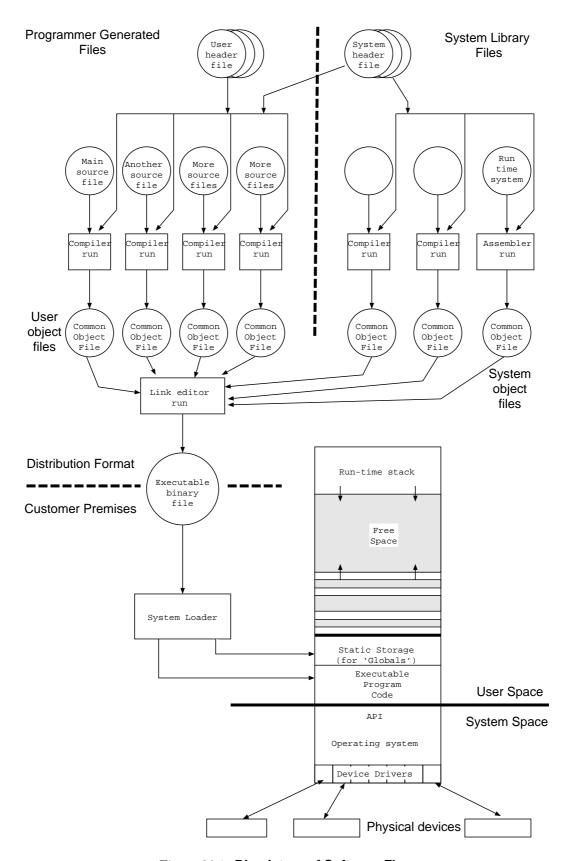
Figure 26.1: Big picture of Software Flow
