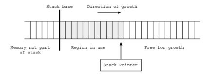
${\rm Figure}~2.2:$  Example of a stack with a number of locations in use
