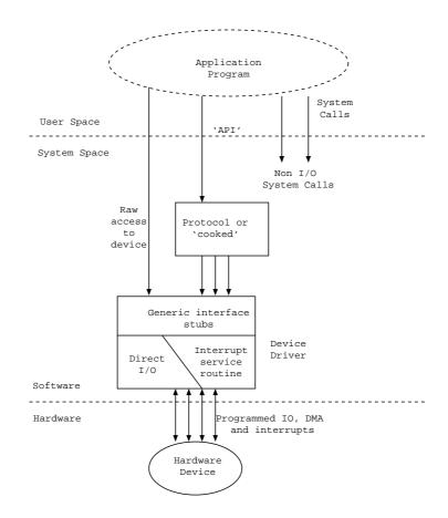
${\rm Figure}\ 17.1:\ \textbf{Device access diagram}$
