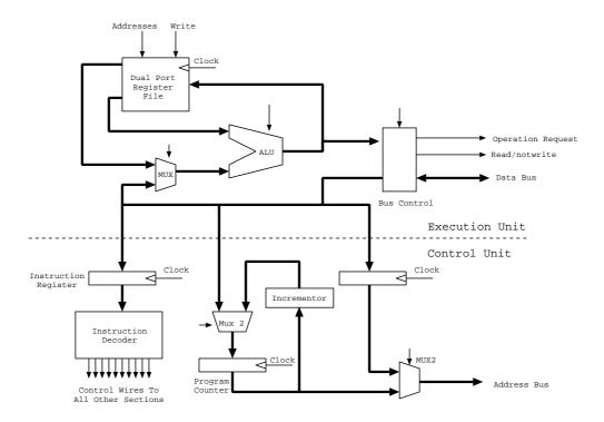
Figure 2.1: Block diagram of a simple microprocessor
