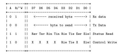
Figure 7.3: Programming model for an example UART
