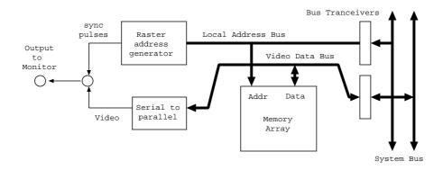
Figure 7.4: Memory Mapped Display Controller Block Diagram
