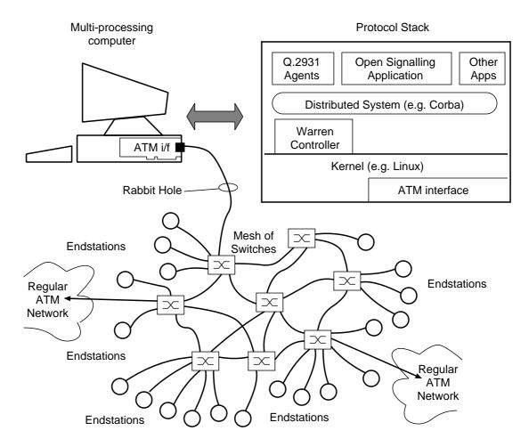
Figure 3: Physical Configuration of an ATM Warren and Protocol Stack within the C ontrol Computer.
