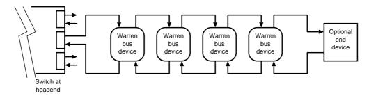
Figure 4: Structure of an ATM bus with an optional regular device on the end. The two directions of flow are normally within the same cable.
