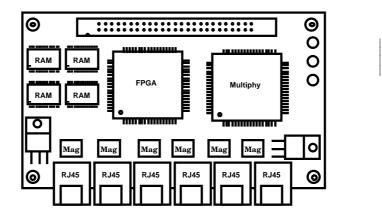
Figure 5: Structure of Warren Switch Version 1 The Version 1 Warren Switch is a six port design with ATM25 on UTP using RJ45 connectors (figure 5). A handful have been built and are in use in Cambridge. This switch is a fully working, standards-compliant ATM switch, but which uses the Warren Control Protocol on a pair of dedicated VCIs, rather than having a processor inside it.
