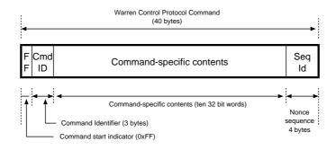
Figure 2: Warren Control Command format within payload.
