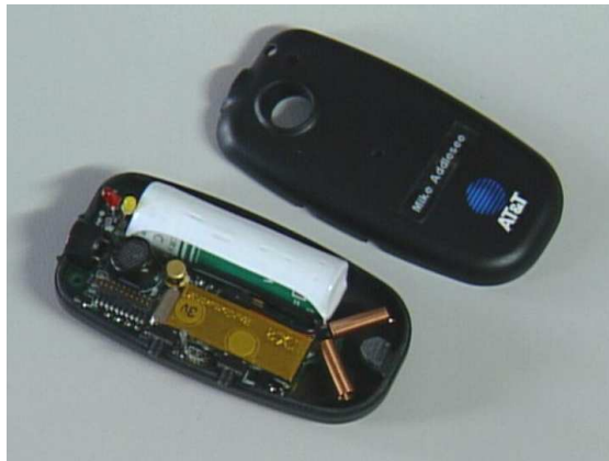
Figure 6.2: One of the wireless tracking tags known as a “Bat”. The device is about the size of a matchbox and features two buttons for input and two LEDs and a sound chip for output. It contains a radio receiver, ultrasonic transmitter, microchip with a unique 48bit ID, and a AA lithium battery supplying enough power for up to 12 months of operation under normal conditions.
