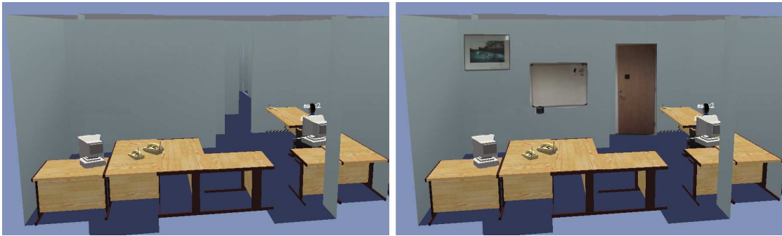
Figure 6.30: Visually augmented representation of the world model. Left: LabView generated view of an office. Right: The rendered scene has been augmented with texture maps acquired from a calibrated camera.
