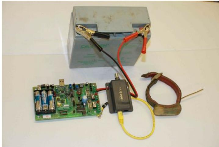
Fig. 3. The badger detection node (left) and the active RFID tag, potted in epoxy and mounted on a collar (right).
