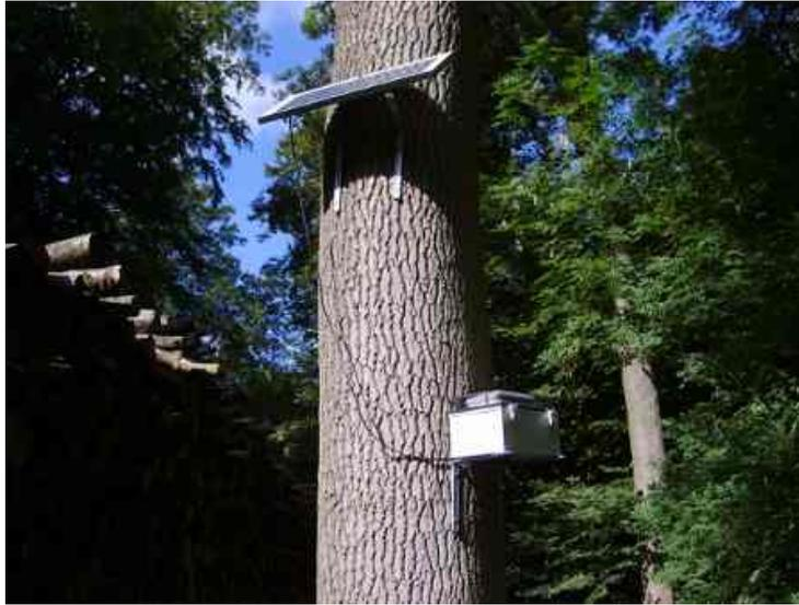
Fig. 6. Deployed 3G Link. The solar panel provides power for the link which is housed within the box on the right-hand side of the picture.
