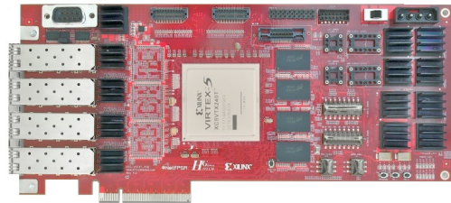
Fig. 4: The NetFPGA-10G board.
