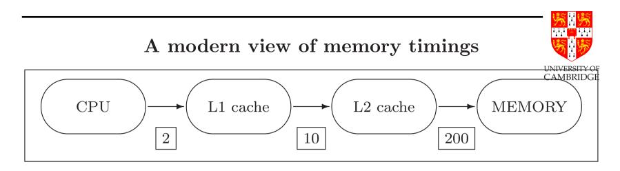
So what happened? On-chip computation (clock-speed) sped up faster (1985–2005) than off-chip communication (with memory) as feature sizes shrank.
