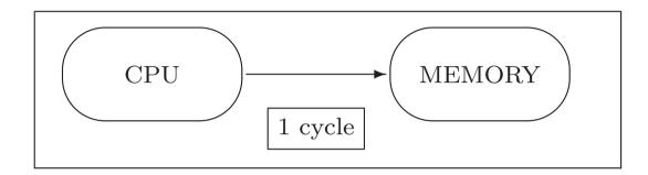
This model was pretty accurate in 1985. Processors (386, ARM, MIPS, SPARC) all ran at 1–10MHz clock speed and could access external memory in 1 cycle; and most instructions took 1 cycle.
