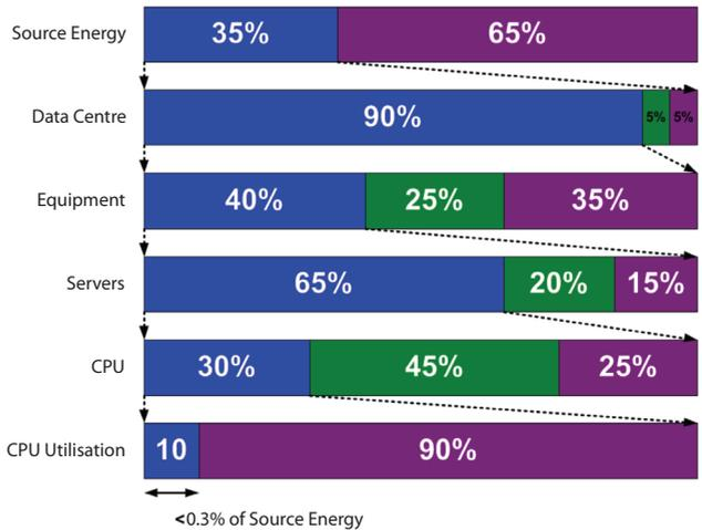
**Figure 2: Diagram showing where energy is lost between source and processor in a 2007 vintage data centre (image courtesy of Liam Newcombe)**
