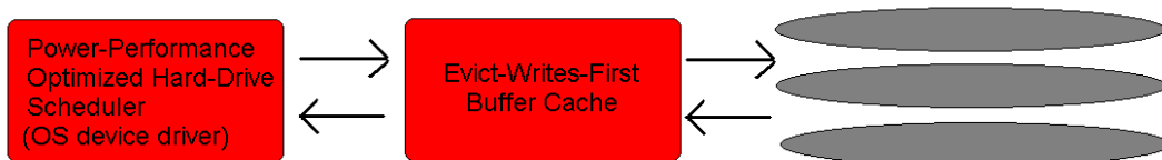
Figure 4: Schematic of optimized hard-drive usage
