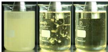
Ultrasonic degassing of oil (5 seconds)
